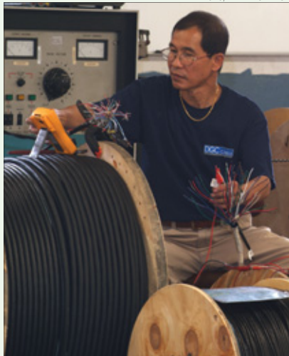
Sean Sorsanavongsa, quality assurance inspector, tests cable for continuity.
