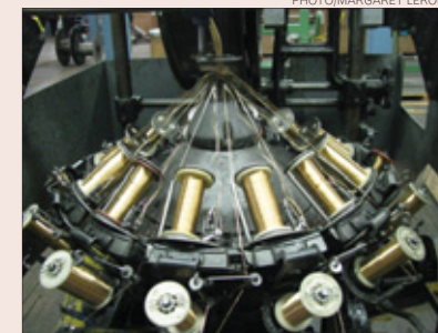
A braiding machine applies a woven bronze shield over cable to prevent external electrical fields from contaminating data in the cable.
